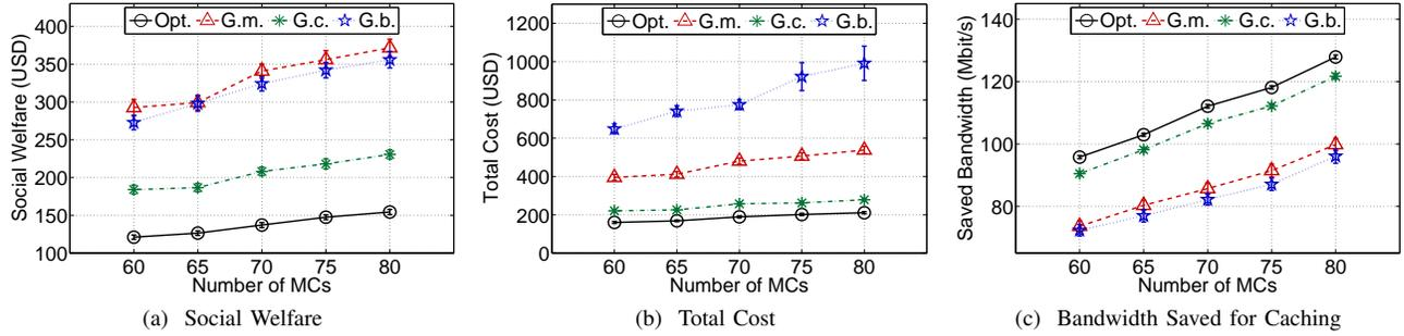
Figure 2. *Social Welfare, Total Cost and Bandwidth Saved for Caching* as a function of the number of mobile clients. The number of access points is set to 50 and the objects cardinality is fixed and equal to  $10^7$ , which corresponds to a Normalized Cache Size  $N$  of 0.524; this means that, on average, caches can store 52% of the total number of objects.
