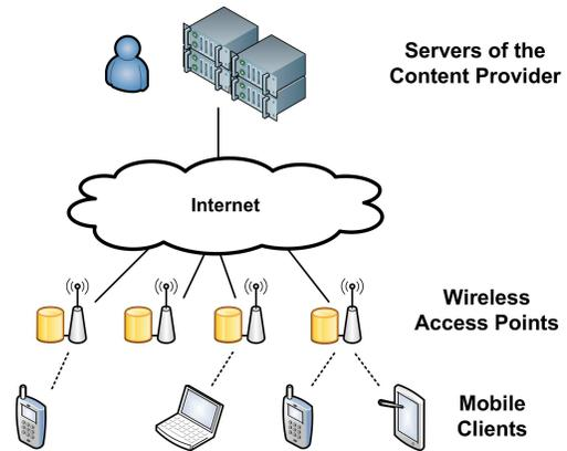
Figure 1. *Network architecture*. A single content provider (CP) is considered in our design. Access points (APs) are equipped with caching storage. Mobile clients (MCs) connect to a subset of the available APs. The demand of a MC will be satisfied either by cached content, or by retrieving the data directly from the servers of the CP using the available backhaul Internet connection. Our mechanism derives the MCs to APs allocation that minimizes the total cost.
